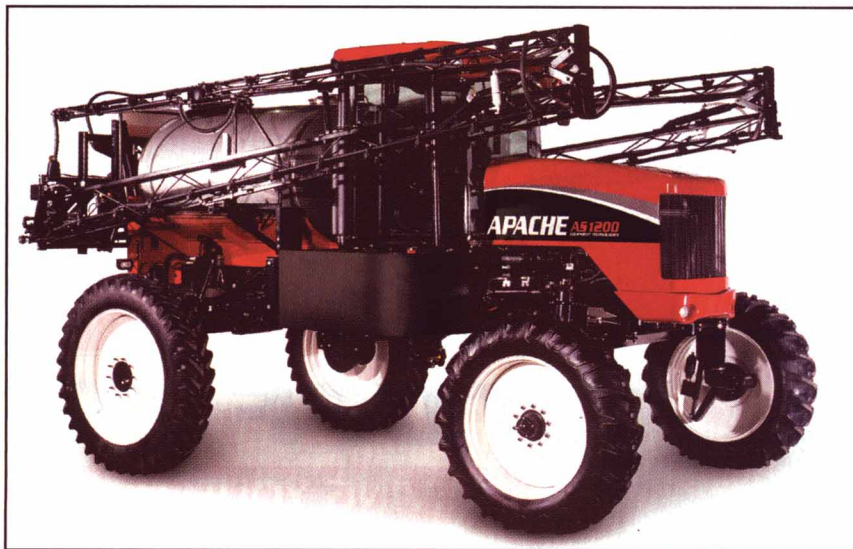
Unlike hydrostatic sprayers which are prevalent in the market, ET's Apache sprayer line is mechanically driven, utilizing ITL and Funk transmissions.
